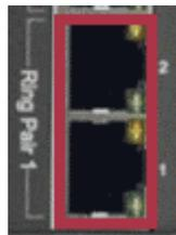
Indicate Ring Pair 1 is enabled (Jumper 6 is “ON”)
